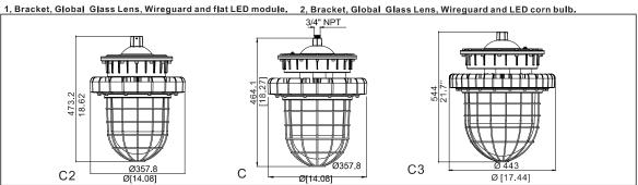
This structure type with bracket, global glass lens and wireguard generates 180° light distribution. We also can put corn bulb In the global glass lens to make this beam angle up to 360°.
