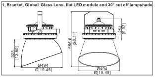
This structure can make the lighting distribution more concentrated for special beam angle.
