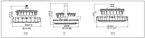
This structure type with bracket, flat glass and optics lens generates 40°,60°,90° and 120° light distribution.
